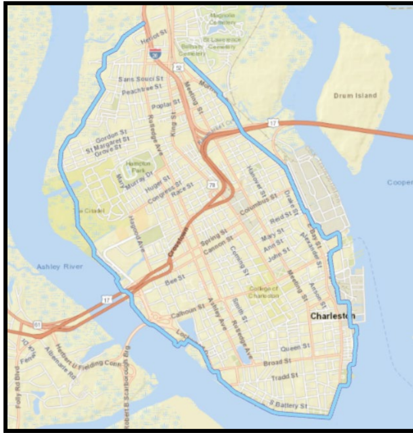
Figure 5.3.3 Alignment of the Perimeter Storm Surge Wall
